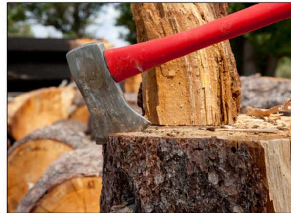
Simple Machine: Wedge
